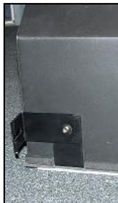
Bracket mounted horizontally
